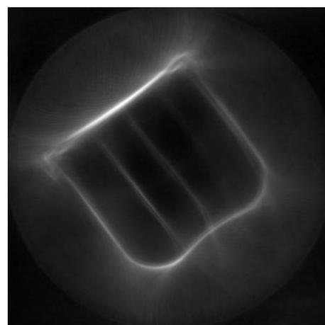
Figure 4. Reconstructed cross section using local sound speeds and absorptions. Contrast and sharpness are increased compared to figure 2. The doubled lines are merged.
