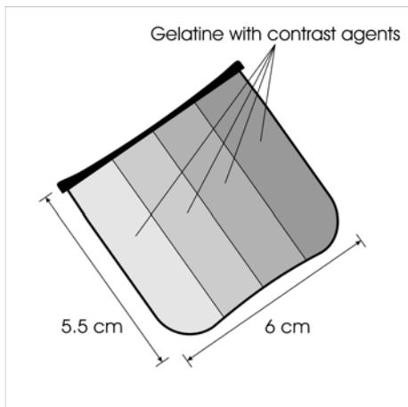
Figure 1. Cross section of the examined ultrasound phantom. It consists of a box with four departments filled with gelatine containing different concentrations of contrast agent.
