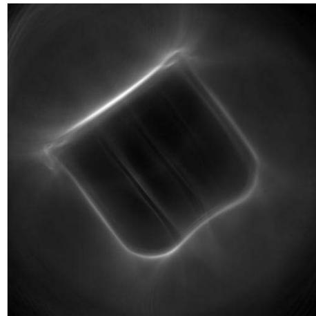
Figure 2. Reconstructed cross section of the phantom. 100 emitting positions with 720 receiving positions each were used for reconstruction. The inner lines appear doubled.
