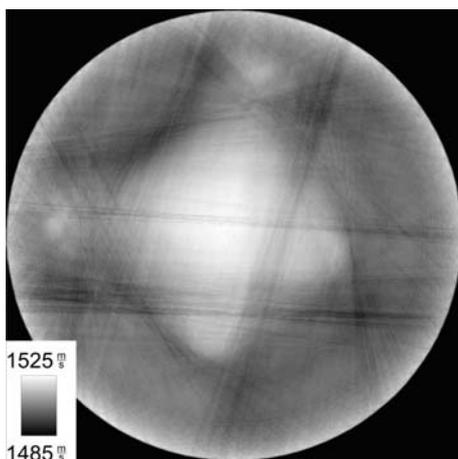
Figure 3. Local sound speeds of the examined phantom. The image was reconstructed using transmission tomography.
