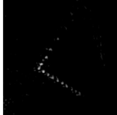
Fig. 1. Reconstructed nylon threads of 0.1 mm in diameter and 0.5 mm distance recorded at 3 MHz with the 2D USCT demonstrator [3].
