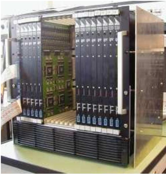
Fig. 2. USCT crate for fast recording of ultrasound data containing several digitization boards (DBs) and one controller board (CB, left with cables).
