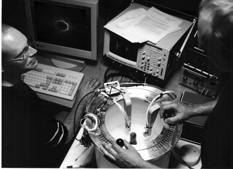
Figure 4. Experimental prototype at Forschungszentrum Karlsruhe. The white tank which is filled with water, contains the object to be examined. Two ultrasound transducer arrays are mounted on rotating rings to simulate all emitter and receiver positions in two dimensions. The signals are digitized, using a digital oscilloscope.
