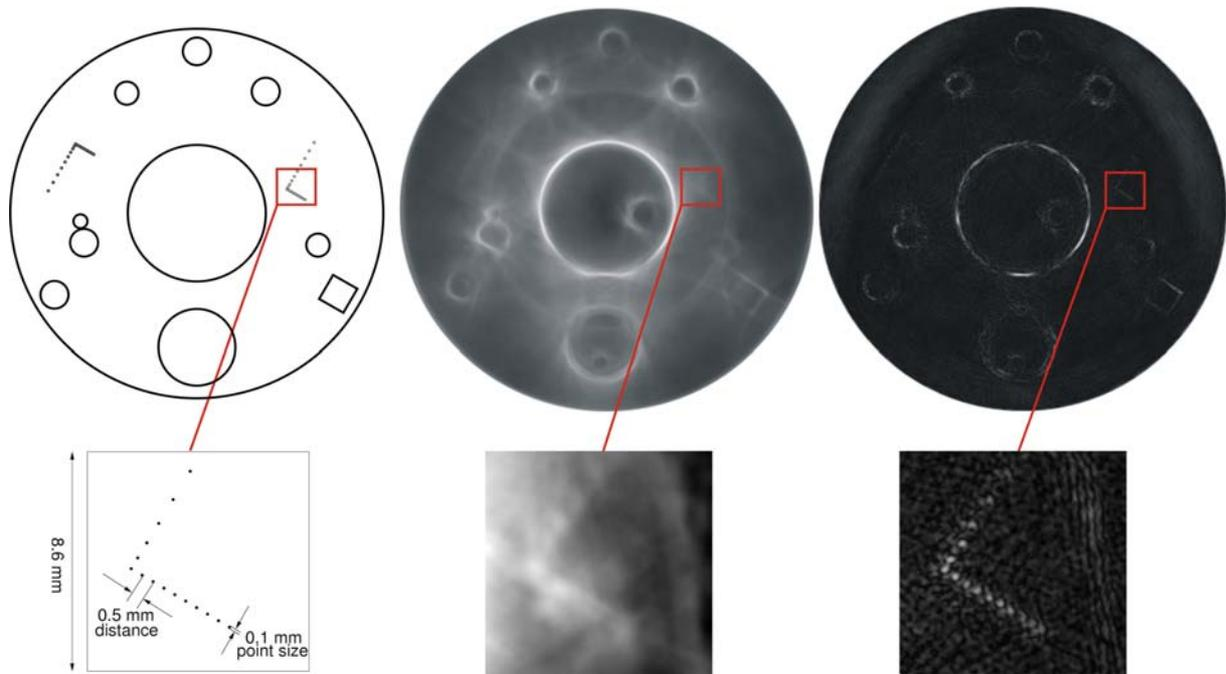
FIGURE 3: Phantom and reconstructed images. Left: Rough plan of the phantom. The diameter is 8.5 cm. The smallest structures consist of nylon threads with a diameter of 0.1 mm and a spacing of 0.5 mm shown in the region enlargement below. Middle: Reconstruction using only amplitude information. Right: Reconstruction including phase information. The nylon threads are clearly visible.
