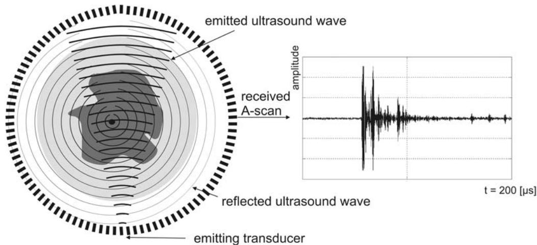
FIGURE 2: Architecture of the USCT system built in our institute, shown in 2D. A ring (cylinder) of ultrasound transducers encloses the object (left). One transducer emits a short ultrasound pulse, all other transducers receive simultaneously. The A-scan at the right side shows the directly transmitted and scattered signals.
