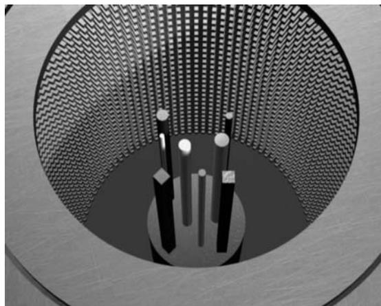
FIGURE 1: Fixed arrangement of transducers for 3D ultrasound computer tomography. The transducers are arranged in a cylindrical array around a tank containing the object and water as the coupling medium.
