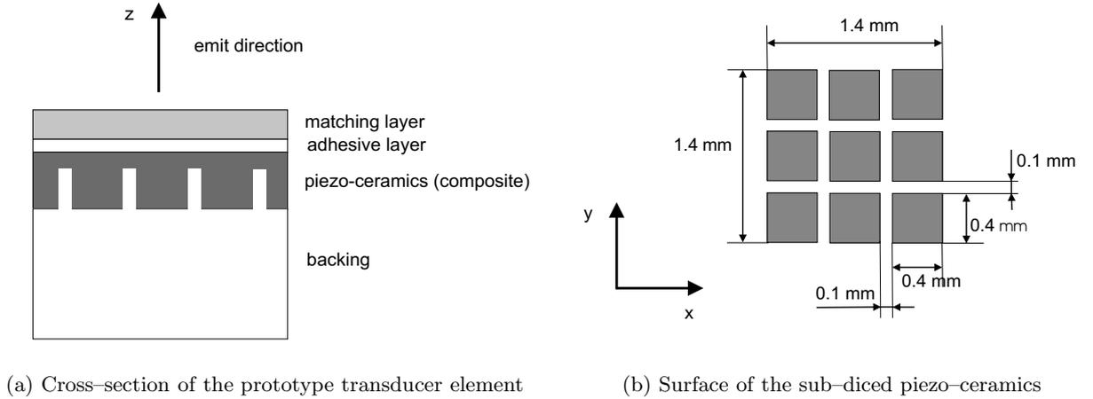
**Figure 4.** Design of the prototype transducer element. Left: cross-section of the sub-diced piezo-ceramics with adhesive layer, matching layer and backing. Right: The surface of the piezo-ceramics is sub-diced in 9 sub-elements.
