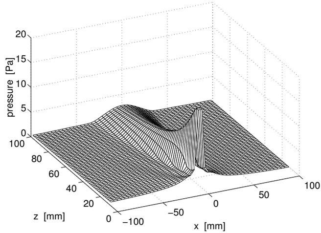
**Figure 6.** Simulated sound pressure in the  $xz$ -plane. The transducer is located in the origin of the coordinate system.
