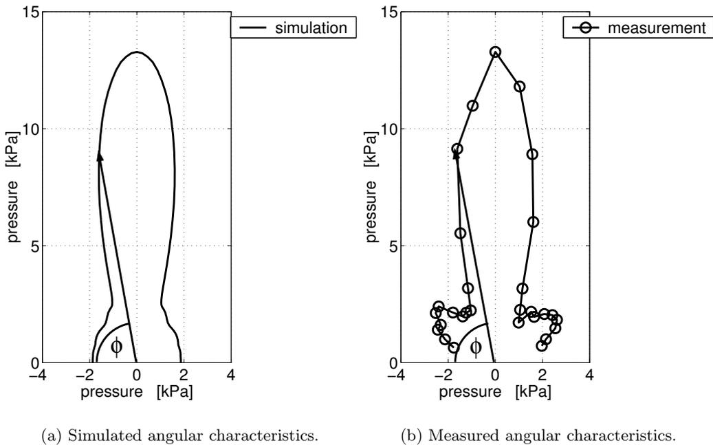
**Figure 7.** Simulated (a) and measured (b) angular characteristics of the prototype transducer element. The distance from the origin to a point of the curve corresponds to the maximum pressure in the direction described by the angle  $\Phi$  as shown in the graphs. Under consideration of the measurement error the simulated and the measured characteristics are almost identical.
