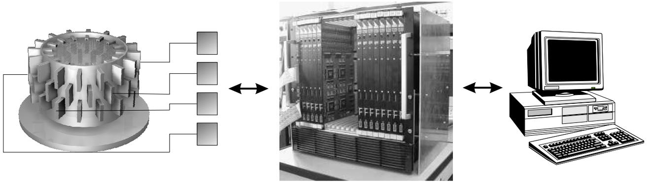
**Figure 9.** Overview of the data recording system. Left: Tank with 48 mounted transducer array systems. Middle: Data acquisition unit with 192 channels. Right: Computer system for image reconstruction.
