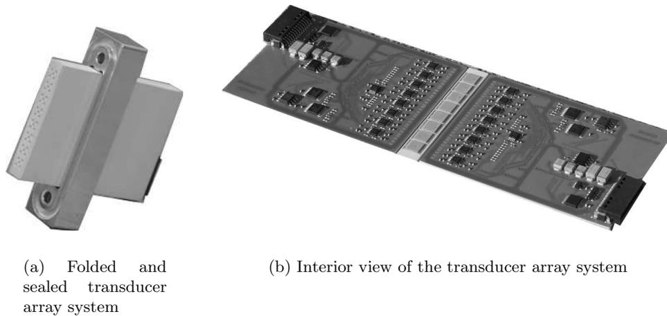
**Figure 8.** Ultrasonic transducer array system with 8 emitters, 32 receivers at the front and integrated controller and amplifier electronics. Figure (b) shows the interior of a transducer array system. The structured piezo-ceramics plate is placed in the center. It is connected to the controller and amplifier electronics at both sides.
