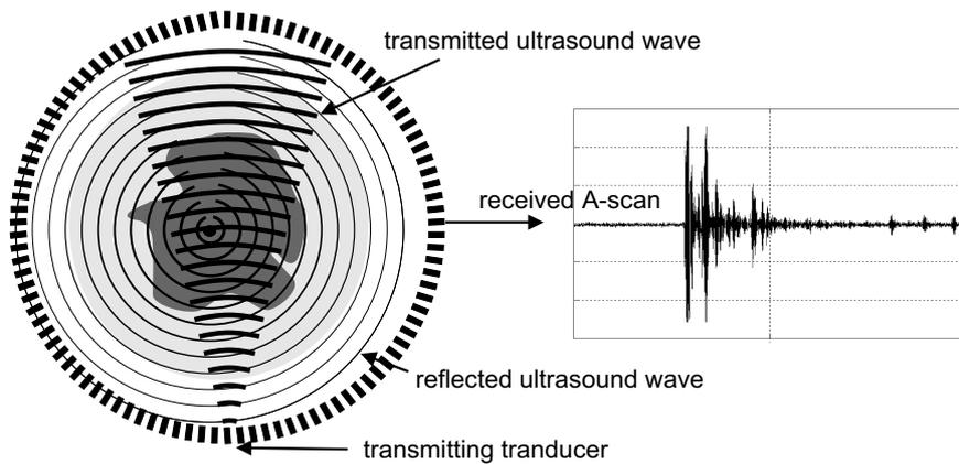
**Figure 2.** Architecture of the USCT system built in our institute, shown in 2D. A ring (cylinder) of ultrasound transducers encloses the object (left). One transducer emits a short ultrasound pulse, all other transducers receive simultaneously. The A-scan at the right side shows the directly transmitted and scattered signals.
