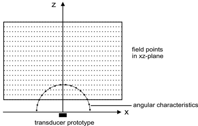
**Figure 5.** Coordinates of the simulated field in the *xz*-plane. The transducer surface is positioned in the *xy*-plane with its edges parallel to the axes. Its center point is positioned in the origin of the coordinate system. The coordinates to measure the angular characteristics are located on a semicircle in the *xz*-plane, radius 20 mm.
