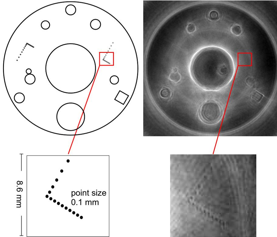
**Figure 3.** Phantom and reconstructed images. Left: Rough plan of the phantom. The diameter is 8.5 cm. The smallest structures consist of nylon threads with a diameter of 0.1 mm and a spacing of 0.5 mm shown in the region enlargement below. Right: Reconstruction using a full aperture sum-and-delay algorithm. The nylon threads are clearly visible.
