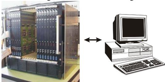
Figure 4: Data acquisition system with 192 parallel channels. The recorded data is transferred to a computer workstation for image reconstruction.
