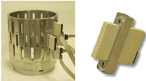
Figure 3: Tank with connected transducer array systems (left) and single transducer array system (right) made in Forschungszentrum Karlsruhe
