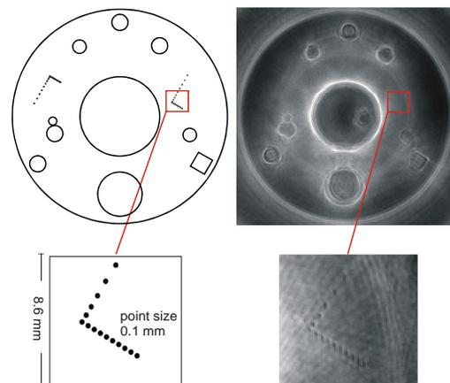
Figure 2: Phantom and reconstructed images. Left: Rough blueprint of the phantom. The diameter is 8.5 cm. The smallest structures consist of nylon threads with a diameter of 0.1 mm and a spacing of 0.5 mm shown in the region enlargement below. Right: Reconstructed cross-section. The nylon threads are clearly visible.
