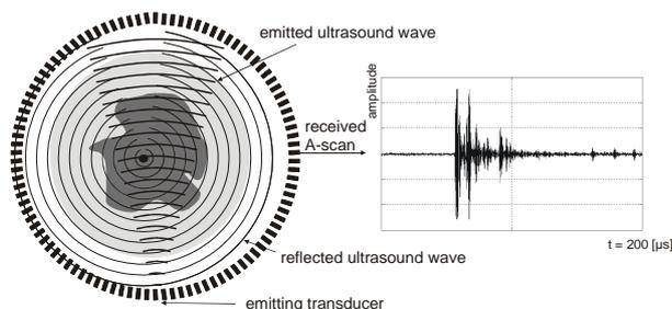
Figure 1: Architecture of the USCT system built in our institute, shown in 2D. A ring of ultrasound transducers encloses the object (left). One transducer emits a short ultrasound pulse, all other transducers receive simultaneously. The A-scan (right) shows the directly transmitted and scattered signals.
